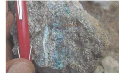
(a) Malachite, azurite, weathering on a monzodiorite piece containing chalcopyrite and bornite.
